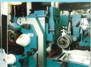
Heavy duty gearbox and cardan drive with central electronic inverter feed drive.
